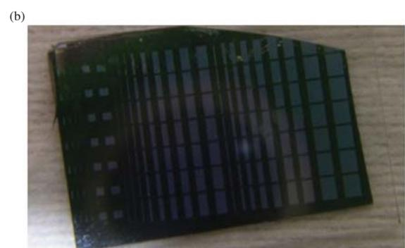
**Figure 4. (a) Mask plate having the Plaza test pattern (b) Plaza test pattern etched 7740 glass substrate**
