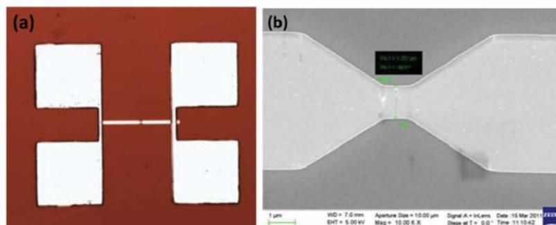
Figure 2. (a) Optical microscope image of the final device (b) SEM image of the notch.
