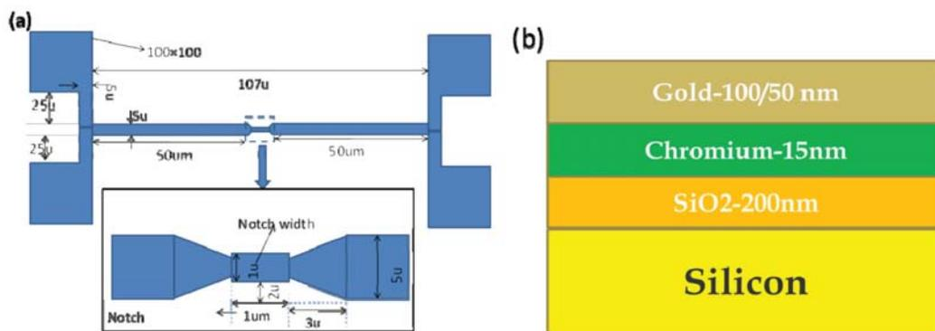
Figure 1. (a) Schematic diagram of the device (top view) (b) layered cross-sectional view with dimensions.
