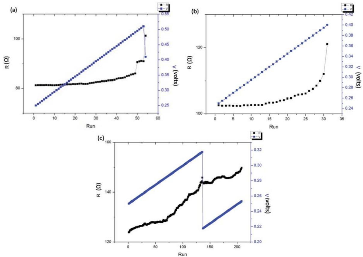
**Figure 7. Variations in driving voltage  $V$  (blue) and resistance  $R$  (black) are shown against the loop number (run); in three steps we reach  $150\ \Omega$  resistance from  $80\ \Omega$  (a)  $80\text{-}100\ \Omega$  (b)  $100\text{-}120\ \Omega$  (c)  $120\text{-}150\ \Omega$**
