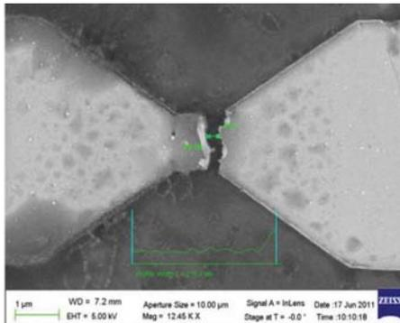
**Figure 4.** SEM image of the device R2C3 after EM.
