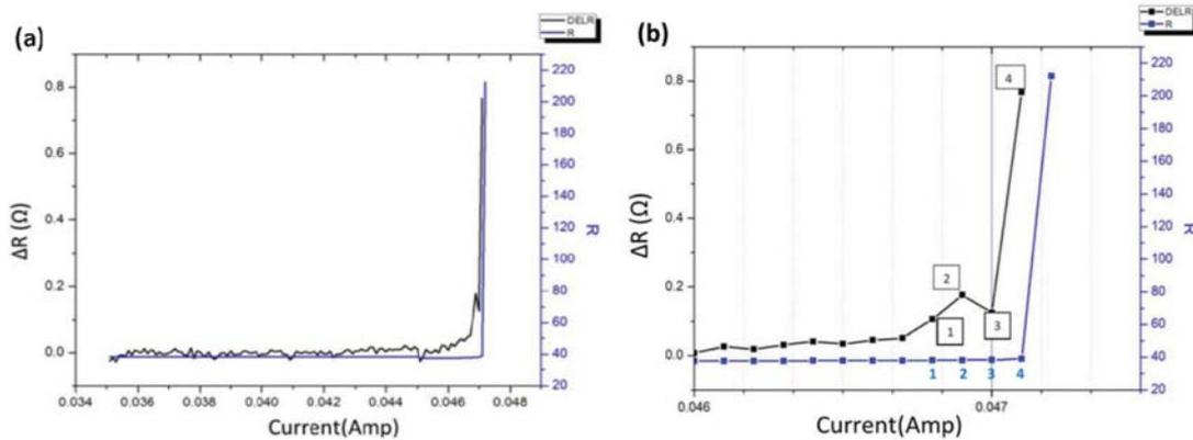
**Figure 3.** (a) Change of R and  $\Delta R$  with increasing current (I) by a ramp rate of 100  $\mu\text{A}/\text{Sec}$ . Here we can see that though the EM occurred at 47.1 mA significant change in  $\Delta R$  only started from 46 mA (b) Enlarged view of Fig. 3(a) (after 46 mA). We can see that EM occurred after data point 4 whereas more than a 10 fold change occurred in  $\Delta R$  from data point 1.
