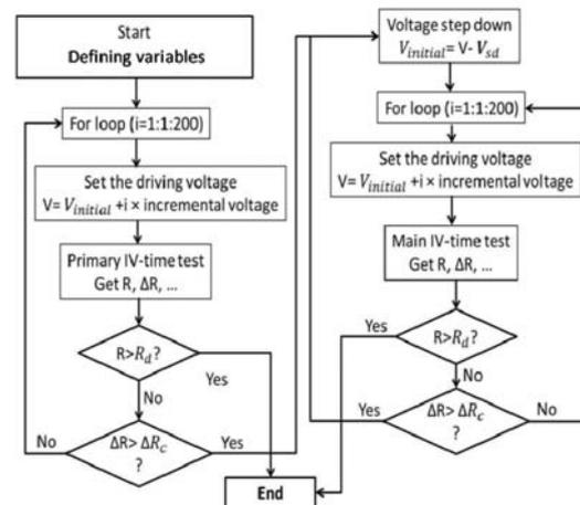
**Figure 5.** Flow chart of Feedback Controlled EM test
