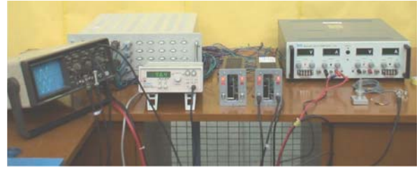
Figure 7: In-flight electronics used to drive the stack actuators
