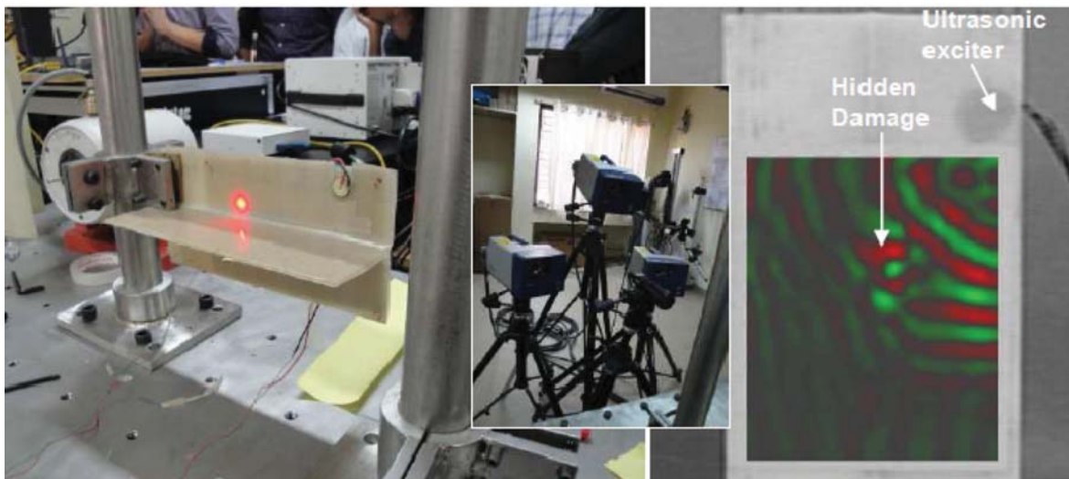
Figure 13. SHM of a composite t-Pull Joint using LDV
