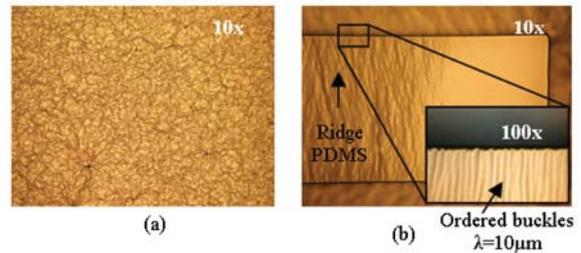
**Figure 1. Microphotographs of sputtered NiCr over PDMS surface: (a) Random orientation of buckles over planar PDMS, (b) Highly oriented buckles over PDMS ridges parallel to the ridge width.**
