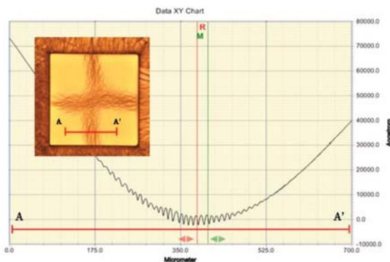
**Figure 2. Variations in buckle wavelength and amplitude from the centre of the ridge to the edges, as obtained from a surface profiler.**
