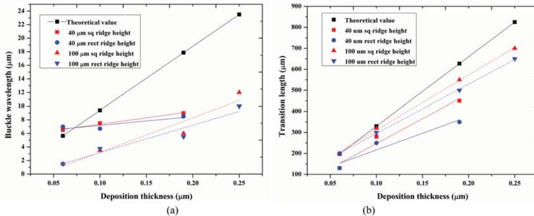
Figure 4. Variation of measured and calculated (a) buckle wavelength and (b) transition length for a film of thickness for 40 μm and ridge height 100 μm, for both square and rectangular ridges.
