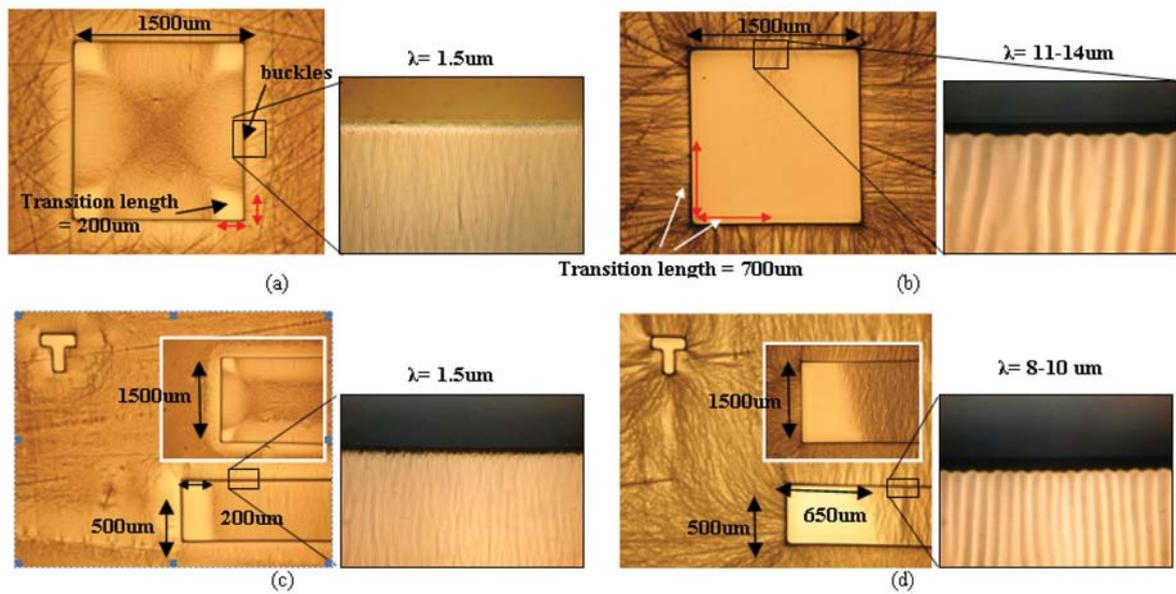
Figure 3. Microphotographs showing variation in buckle wavelength and transition length for the deposition of nichrome over 100 μm height square ridges for (a) 2 min and (b) 15 min and, rectangular ridges for (c) 2 min and (d) 15 min. The inset of (c) and (d) shows corresponding rectangular ridges of width 1500 μm.
