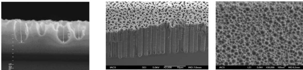
Fig.1 Different micro/nano structures fabricated by electrochemical etching
