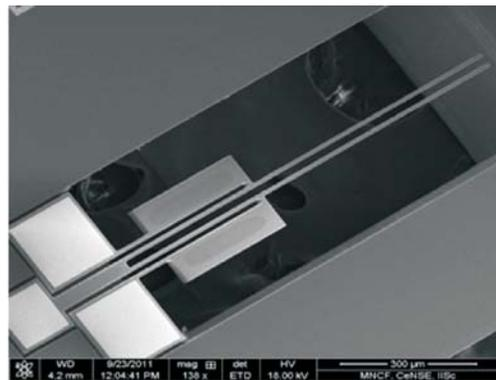
Fig 1 SEM picture of the Micro Tweezer
