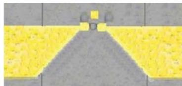
Fig.4a Cell trapped between elliptical electrodes touching both the walls on the upper side
