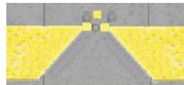
Fig.4b: Cell trapped between elliptical electrodes touching both the walls on the lower side
