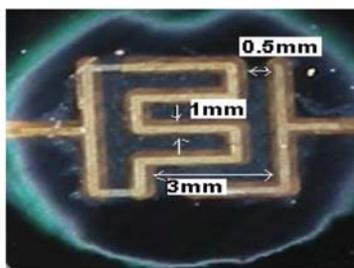
Fig.2a Functionalized microchannel sensor for bacteria detection
