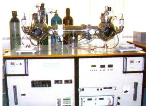
Fig. 1. RF/DC magnetron sputtering system
