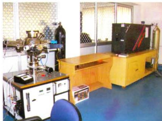
Fig. 2. Pulsed laser deposition system
