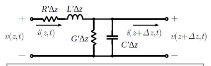
$$-\frac{\partial}{\partial z}v(z,t) = R'\ i(z,t) + L'\ \frac{\partial}{\partial t}i(z,t)$$
