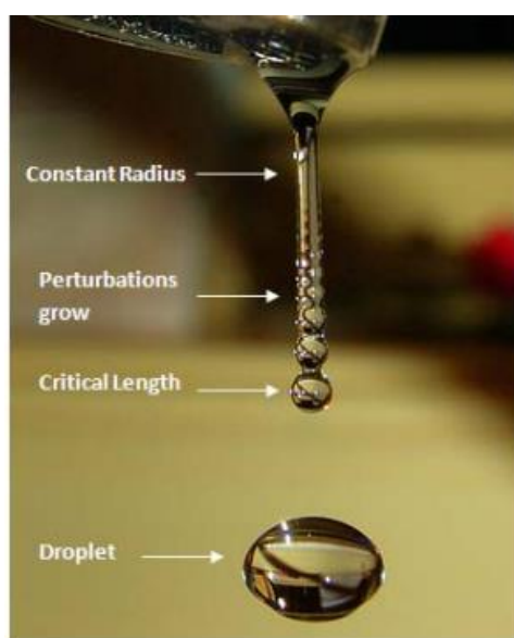
Breakup of a liquid jet
